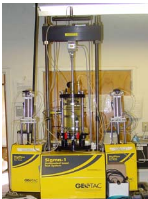
K_0 System with Flow Pumps
